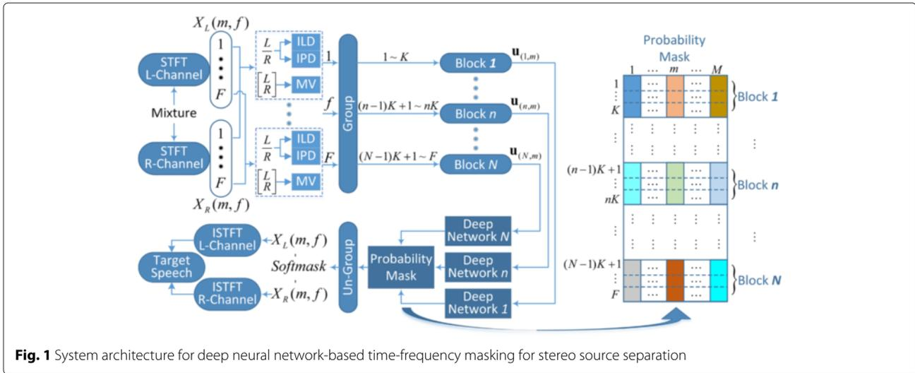
**Fig. 1** System architecture for deep neural network-based time-frequency masking for stereo source separation
