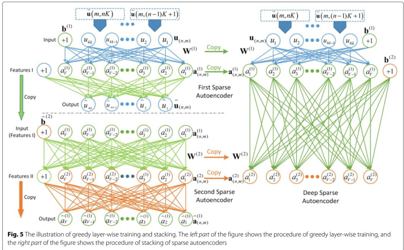
**Fig. 5** The illustration of greedy layer-wise training and stacking. The left part of the figure shows the procedure of greedy layer-wise training, and the right part of the figure shows the procedure of stacking of sparse autoencoders
