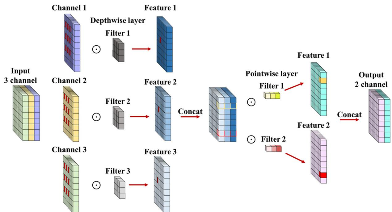
Fig. 3 Block diagram of the depthwise separable convolution with dilated filter in DDC-block
