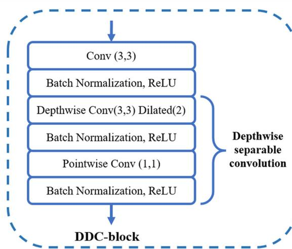
Fig. 2 The internal structure of DDC-block module
