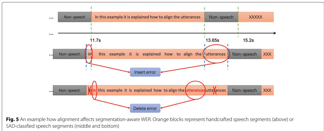
**Fig. 5** An example how alignment affects segmentation-aware WER. Orange blocks represent handcrafted speech segments (above) or SAD-classified speech segments (middle and bottom)
