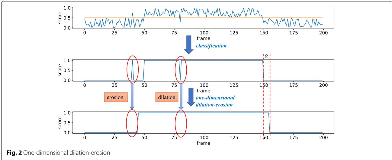
Fig. 2 One-dimensional dilation-erosion
