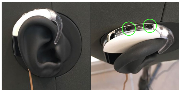
Fig. 2 Dummy BTE pieces used for creating the database. Each BTE piece consists of two omnidirectional microphones as indicated by the circles
