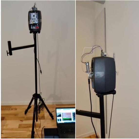
**Fig. 3** Hardware setup for experiments with single channel microphone-loudspeaker
