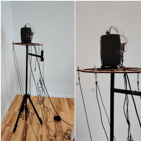
**Fig. 4** Hardware setup for experiments with multi-channel microphones organized in a uniform circular array with a loudspeaker placed at the center of the array
