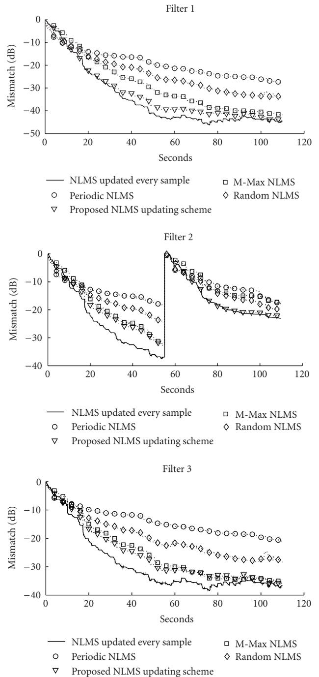
FIGURE 5: Mismatch for the the evaluated methods, where an echo-path change occurs for filter 2 after 55 seconds.
