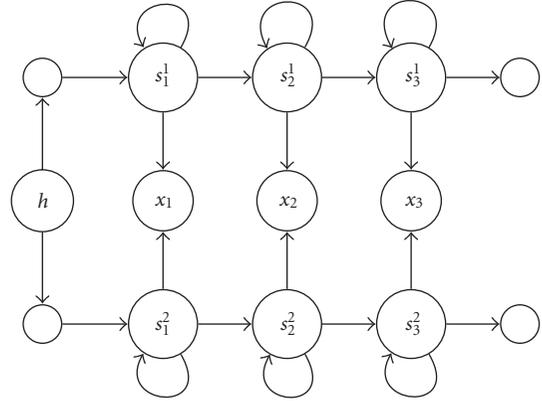
FIGURE 4: A phoneme mixture model. The generating model depends on the hidden variable  $h$ , which determines the mixing coefficients between model 1 and 2. The random variable  $h$  in general depend on other variables. The distribution of the observation is a mixture between the two distributions predicted by the two hidden models, mixed according to the mixture model  $h$ .
