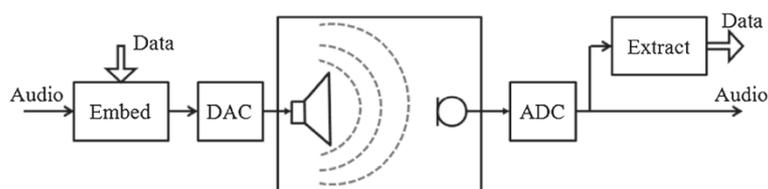
**Figure 12** Embedded data transmission over acoustic channels.
