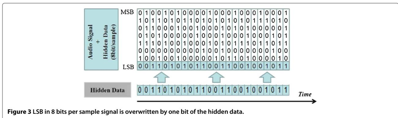
**Figure 3** LSB in 8 bits per sample signal is overwritten by one bit of the hidden data.
