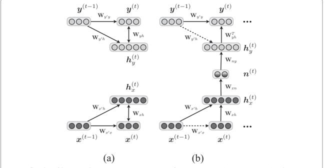
**Figure 1 A flow chart of the proposed voice conversion system. (a)** CRBMs for a source speaker (below) and a target speaker. **(b)** Our proposed voice conversion architecture combining the two pre-trained speaker-dependent CRBMs with a concatenating NN.
