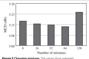
**Figure 5 Changing mixtures.** The values show averaged Mel-cepstral distortion with varying numbers of mixtures M for GMM method (N = 20,000).
