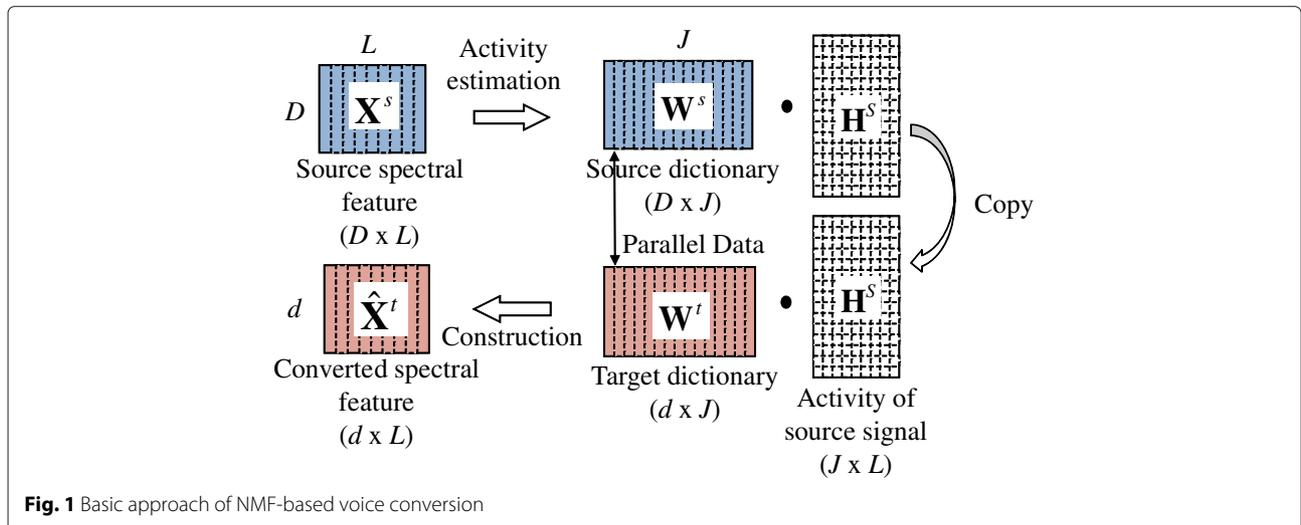
Fig. 1 Basic approach of NMF-based voice conversion
